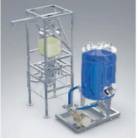
Conti-TDS module with process vessel on load cells and powder addition from a big bag station
