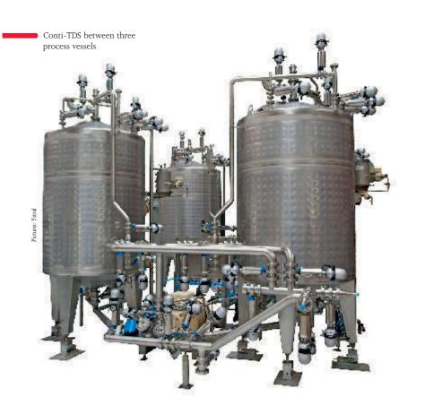
hopper or container. The dust-free induction is one of the key arguments to use that system. No powder is poured onto the surface of the liquid. No bag has to be lifted on top of the vessel. No dust sticks to the inner wall of the tank, and no powder is emptied onto the surface of the liquid in the presence of solvent vapour.
