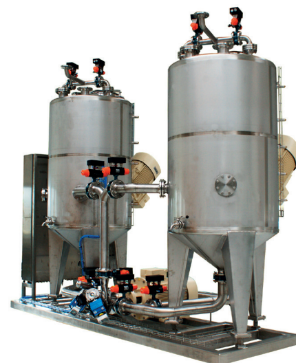
Figure 5. Skidded unit with one Conti-TDS-5 between two process tanks
