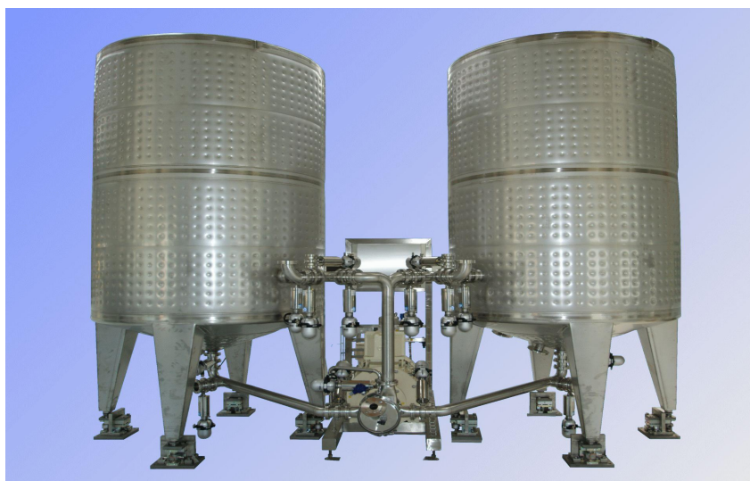
Fig. 1: ystral Conti-TDS with a Big-Bag-Station between two process tanks
