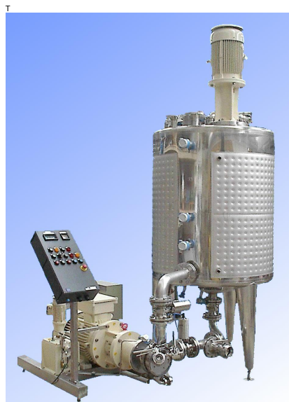
Fig. 8: ystral Conti-TDS in a system for varying batch sizes.
