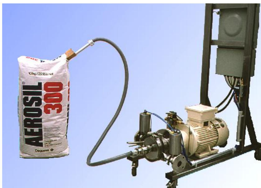
Fig. 3: ystral Conti-TDS with induction tube for the dust-free incorporation of fine powders
