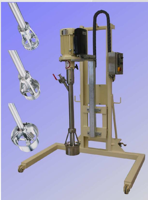
**Multipurpose machine with moveable lift, quick coupling and exchangeable tools**
